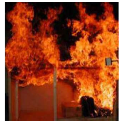
EN 13501 PART FOUR : EN ISO 9239 1 - WIND OPPOSED HORIZONTAL SPREAD OF FLAME
