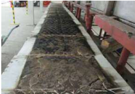
CORE AFTER TEST (LOCATED NEAR THE FIRE END)
