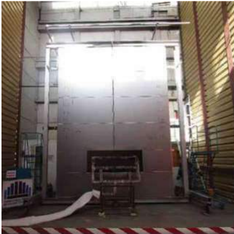
NFPA 285 PANEL FACES PRIOR TO FIRE TEST
