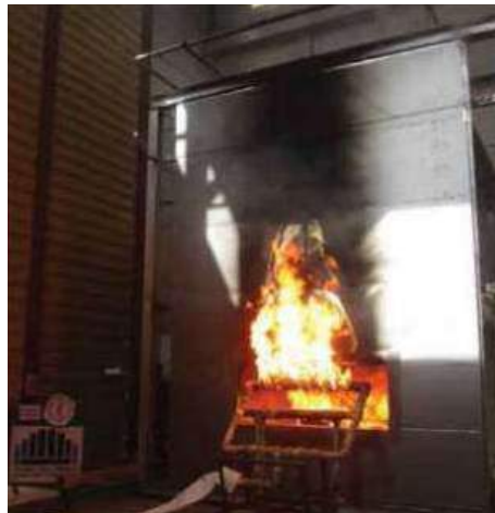
EXTERIOR FACE AT 25 MINUTES OF THE TEST
