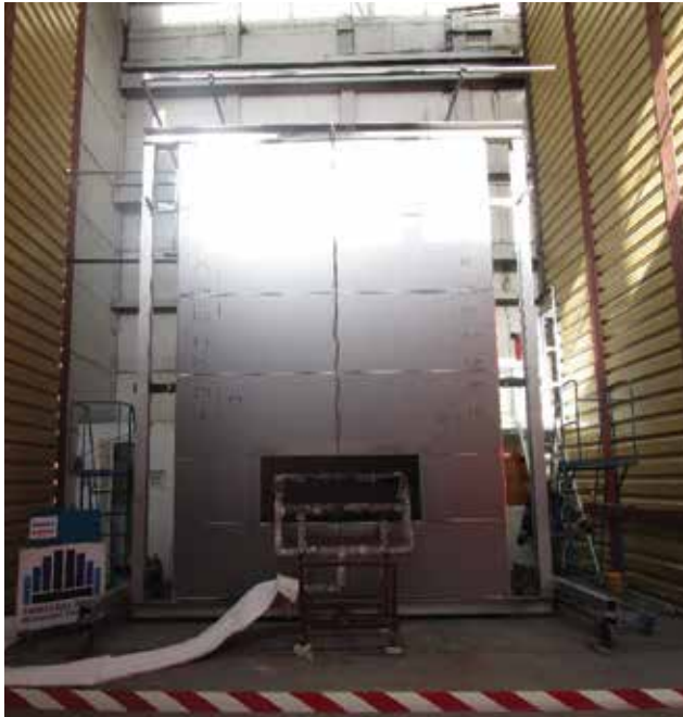
NFPA 285 PANEL FACES PRIOR TO FIRE TEST.
