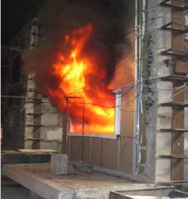
FULL FIRE IN BOTH FLOORS - TEMPERATURE 850 °C
