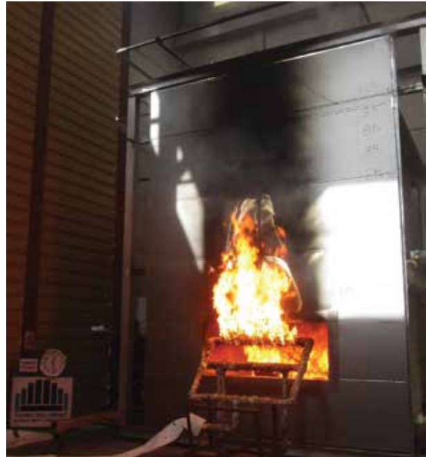
EXTERIOR FACE AT 25 MINUTES OF THE TEST.
