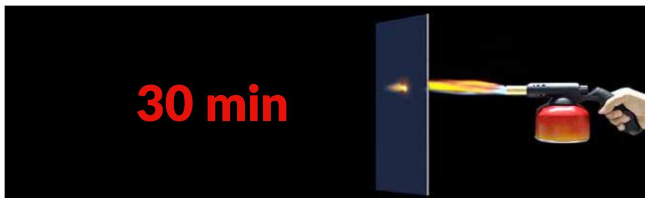
A2 MINERAL CORE - ACP PANEL - FIRE PENETRATED IN 30 MINUTES
