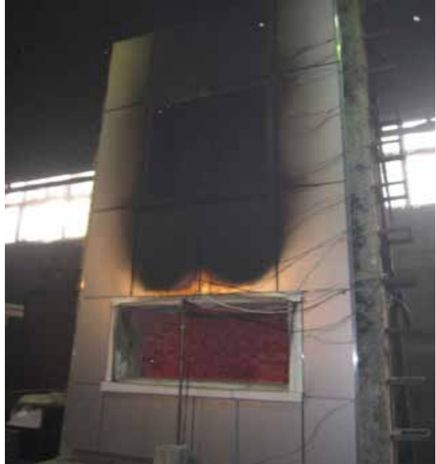
FIRE STOPPED AFTER 60 MINUTES ALL PANELS WITHOUT DAMAGE
