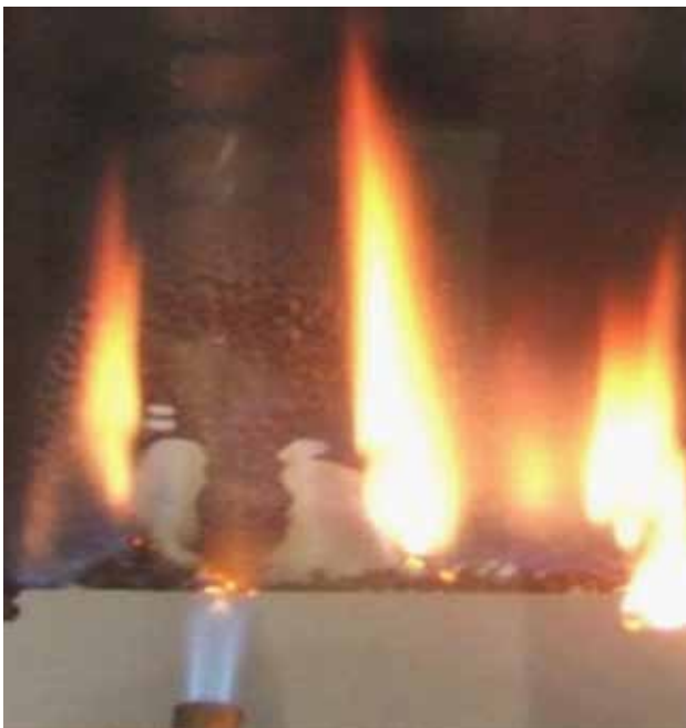
EN 13501 PART THREE : SMALL FLAME ATTACK
