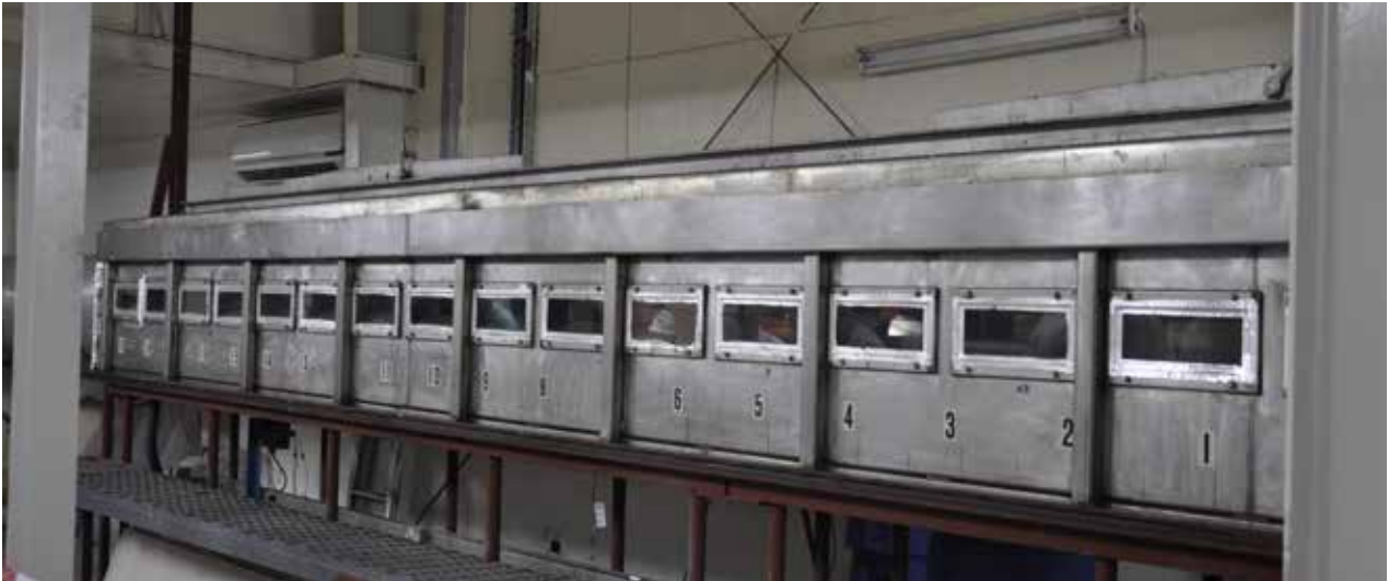
STEINER TUNNEL FIRE MACHINE
